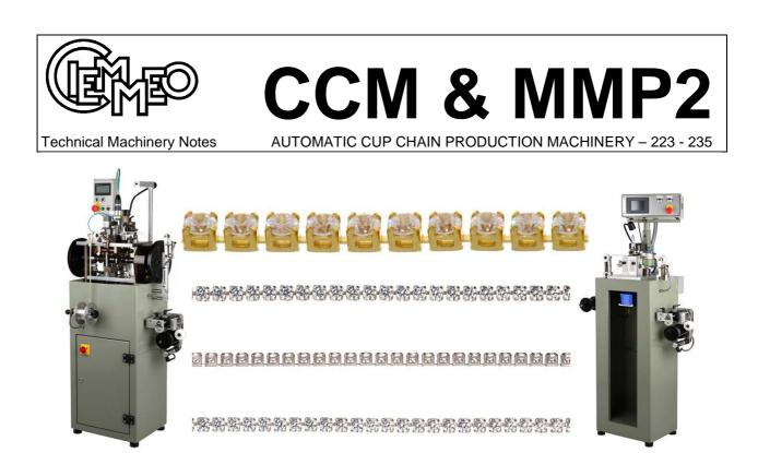
Two fully automatic machines which complement each other for the production of high quality cup chain. Flat calibrated strip is fed to the CCM which stamps the individual cup and its connecting rod. Assembly of the two pieces is carried out continuously forming а uniform chain of empty cups
