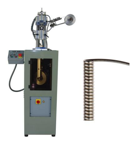
Part of the Spring Ring production line, the MFS is an automatic machine which sees to creating a continuous spiral of cored hollow tube.
