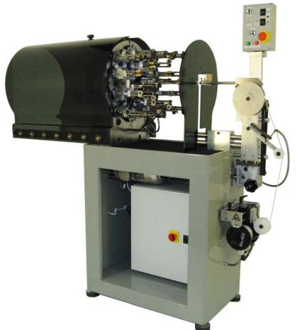
amount of strands may be used (up to a max. of 16) to create different braid textures. Braid inclination angle and drawing speed are manually adjustable
