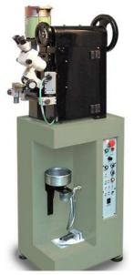
The soldering of the links together is carried out directly on the ATMC assembling machine. A laser with a patented focusing head solders the links together internally so that no soldering can be seen on the chain itself. The weld is a full weld, therefore not requiring any further soldering treatment.
