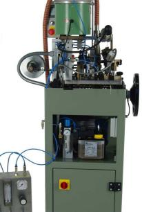
Part of the Spring Ring production line, the MSSA is a sophisticated machine which sees to creating and then automatically soldering an endring to the Spring Ring housing.
