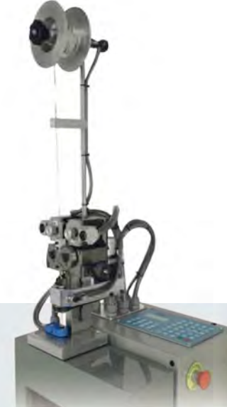
Basic automatic programmable twisting machine. Able to transform chains by twisting in all directions, continuously and alternatively.
