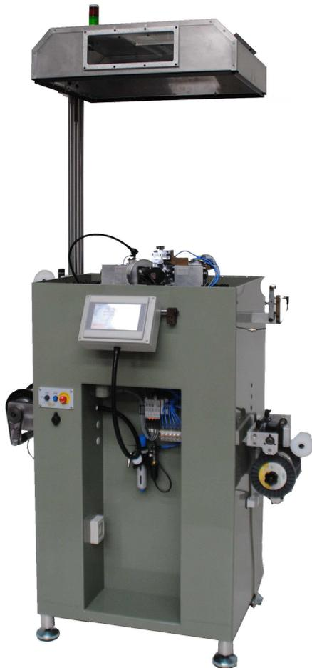
Optic fibres handle communication between the PLC and the synchronised brushless motors, which allow micrometric precision in positioning and speed.
